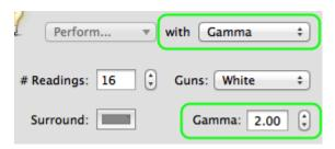
Assuming you have access to a supported *photometer* (for example a **i1** or **Spyder** device), select it and the readings will be automatically sent to Psykinematix as you take the measurements. If your *photometer* is not in the list of supported devices, then it is still possibe to use it by entering manually its luminance readings. In this case, select the **Readings** option.
