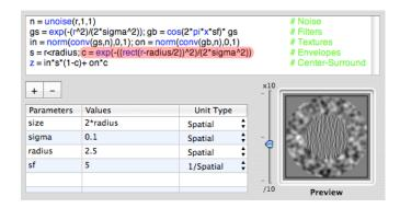
To perform this operation, one computes the distance to the inner boundary for each pixel beyond it, to which is applied the Gaussian modulation: **rect** ( $\mathbf{r}$ -radius/2) returns this distance if  $\mathbf{r} >= radius/2$ , and 0 otherwise.
