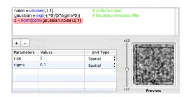
Note that the convolution function is performed using a highly optimized fast Fourier transform (FFT) algorithm.
